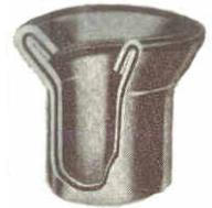
\* NOTE: ONLY DOUBLE WALLED SEAMLESS STEEL LINES WITH DOUBLE FLARED ENDS ARE APPROVED FOR BRAKE LINE APPLICATIONS — COPPER TUBING AND SINGLE WALL BUTT WELD STEEL TUBING IS NOT APPROVED
