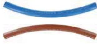
**PFT-FL** - Nylon. Heat and light stabilized for use in tractor, trailer and other mobile diesel fuel systems. Working pressure up to 150 psi. Sizes 1/4" - 3/4" O.D. -40°F to 200°F. Blue. **HTFL** - Polyamide. Heat and light stabilized for use in mobile diesel fuel systems. Working pressure up to 175 psi. Sizes 3/8" - 3/4" O.D. -50°F to 266°F. Brown.
