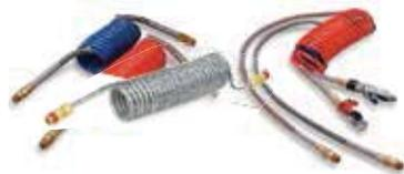
**Brakcoil®, DuoCoil™, DollyCoil™, SliderCoil™** Coiled nylon tubing for tractor-to-trailer air brake systems. Available in pre-assembled kits for easy installation. Color coded - Blue for service, Red for emergency. Working lengths to 15 feet. Up to 150 psi. Sizes 1/2" O.D. **Fifth Wheel Slider Coil** - Nylon. Self adjusting, pneumatic tubing coils. Up to 150 psi. Size 1/4" O.D. only.
