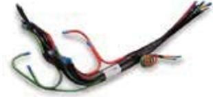
**Harnesses & Bundles** - Custom-engineered air brake tubing harnesses. Used on truck and bus production lines to cut production time and tube scrap. Supplied with pre-cut and pre-formed tube and assembled into a single unit. Sizes 1/8" - 3/4" O.D. For details, view BUL. 4660-Harness.
