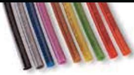
**1120 Type A/B** - Nylon. For mobile air brake and air accessory systems. 100% pressure tested. Working pressure up to 150 psi. Sizes 1/8" - 3/4" O.D. -40°F to 200°F, dependent on type. Meets or exceeds SAE J844 & D.O.T. FMVSS 49CFR571.106 requirements.
