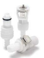
**PPM & PPL Series Couplings** are general purpose, thermoplastic couplings. The push-to-connect feature and push-button release provides simple one-handed operation. The couplers and nipples are available with or without valves. Standard seal material is Nitrile. Applications include:
