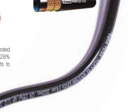
XDH Hose - Designed to be heat formed into custom routings. XDH blends the rigidity of steel tube with the flexibility of a rubber hose. Parflex XDH hydraulic hose is built for high volume, repeatable applications in extreme environmental conditions such as high temperatures, complicated routings, high abrasion, and aggressive fluids. Up to 5,000 psi. -65°F to + 300°F. Sizes 1/4" - 1/2" I.D.
