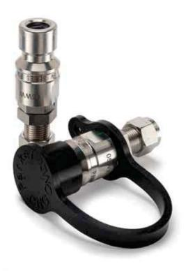
Parker FMS Series receptacles are designed for rigid mounting on a compressed natural gas vehicle. Receptacles can be employed in both fast-fill and time-fill dispensing applications. The ANSI/NGV1 standard used by FMS Series receptacles allows vehicle fueling to be accomplished with all CNG nozzles conforming to the ANSI/NGV1 standard.
