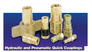
Double shut-off, single shut-off, and non-valved quick couplings are available for hydraulic and pneumatic service. Body materials include steel, stainless steel, brass and thermoplastics and are available in sizes from 1/8" to 2 1/2" (3mm to 64mm). Pressure range up to 10,000 psi (69 MPa). All applicable industry interchanges are available including the proposed ISO 16028 standard for non-spill couplings.
