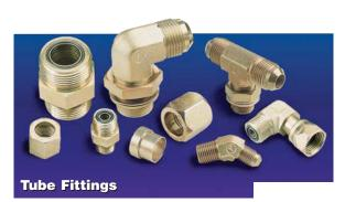
A wide variety of hydraulic tube fittings are available for all types of plastic processing equipment. Products include medium to high pressure Triple-Lok® 37° flare and Ferulok® bite-type fittings. Sizes range from 3/16" to 2" (5mm to 51mm). Seal-Lok® O-ring face-seal fittings are available in the same size range for more demanding high pressure applications up to 6,000 psi (42 MPa).
