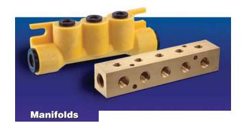
$1/8\H$  to  $3/8\H$  NPTF inlet and outlet ports. Pressures up to 1000 psi. Temperature range from -65°F to +250°F. Convenient junction for multi-branch distribution lines.
