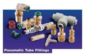
Low to medium pressure up to 300 psi. Temperature range -20°F to +275°F. Sizes from 1/8" to 5/8", 4mm to 14mm O.D. Products feature push-in, compression and barb connection for a wide range of applications.
