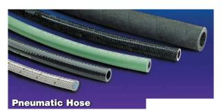
Vacuum to 350 psi (2,4 MPa). Sizes from 1/8" to 1" (3mm to 25mm) I.D. in both rubber and thermoplastic product offerings. Products provide good flexibility and high abrasion resistance for a variety of pneumatic applications. Material options include rubber, thermoplastic, and Teflon®.
