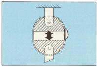
High strength: 100 lb. (445N) and 250 lb. (1112N) minimum loop tensile strength per MIL-S-23190
